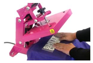
Align the transfer material on the garment to be printed.
