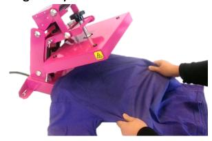
Once the Craft Press has reached the designated temperature, position the garment on the lower platen.
