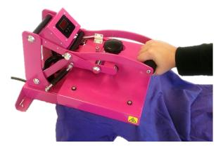
Lower and lock the heat platen into the press position. The automatic timing process will start.
